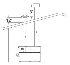
FIG. 16 Roof Top Combustion Air Inlet
